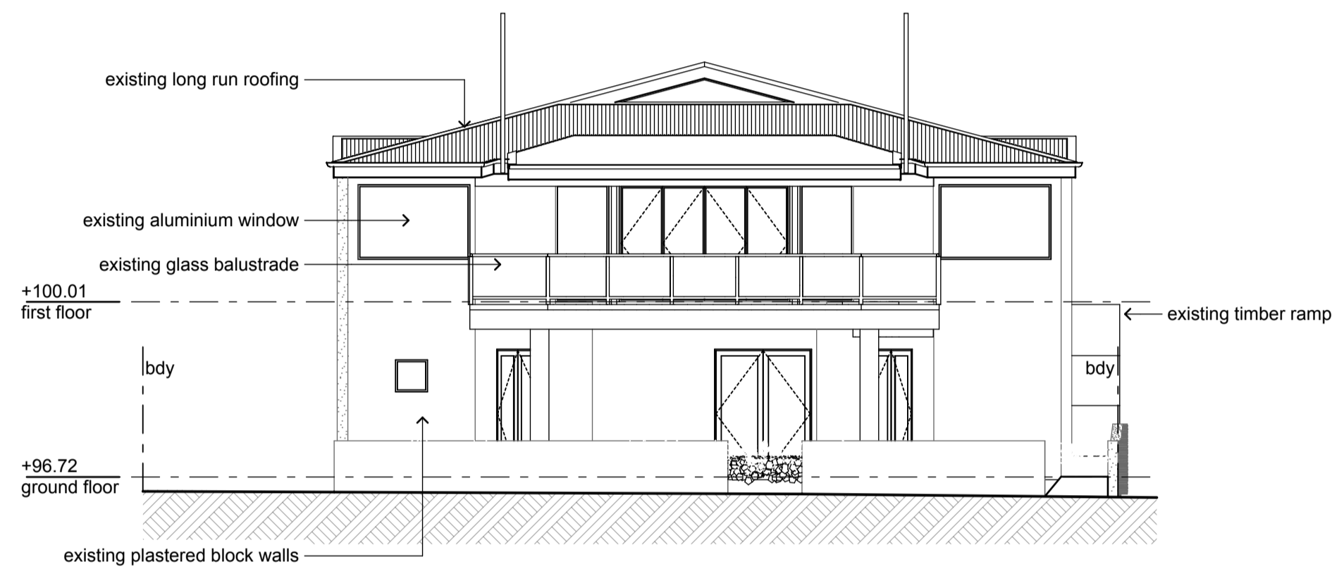
existing west elevation 1:100
