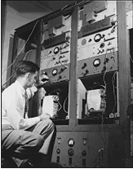
Figure 11 Gordon Stanley, in 1952 January, with the receivers that he developed for the 4.9-m dish and the short-lived 8-Yagi array (ATNF Historic Photographic Archive: 2650–1).
