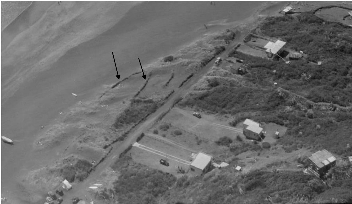
Figure 9: Photograph of Piha taken in January 1951 to the immediate north of the surf club showing brush fences (examples arrowed) erected to control wind erosion. (Whites Aviation photo – from Alexander Turnbull Library).
