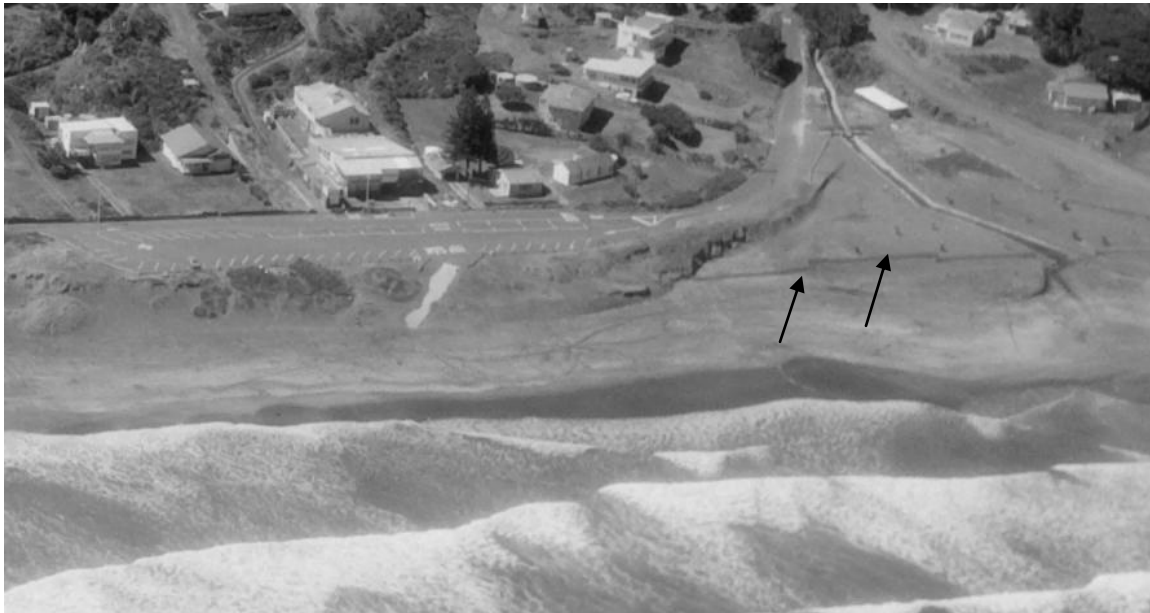
Figure 12: View of surf club car park and Moana Stream entrance area in 1985. Note the concrete stream training works in the Moana Stream and the placement of sand trapping fences (arrowed) to create dunes on the immediate northern side of the former embayment.
